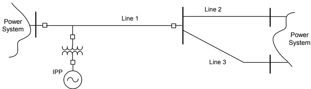
**Figure 13** Transmission Line Connected IPP
