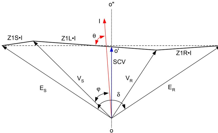
**Figure 8** Voltage Phasor Diagram of a Two-Source System
