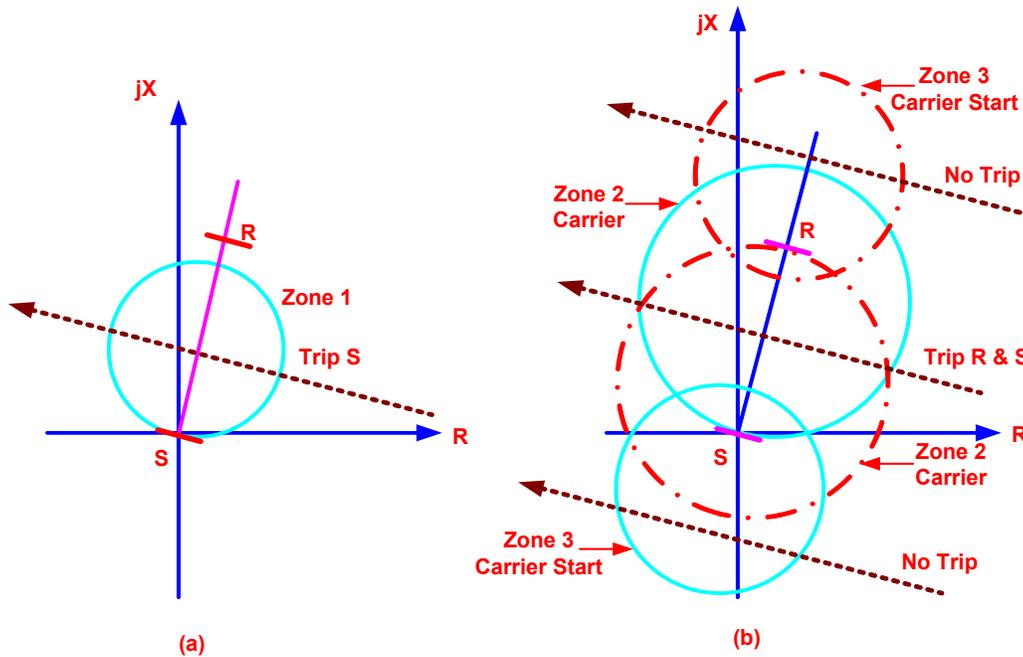
**Figure 1** Zone 1 and Directional Comparison Blocking Scheme Characteristics
