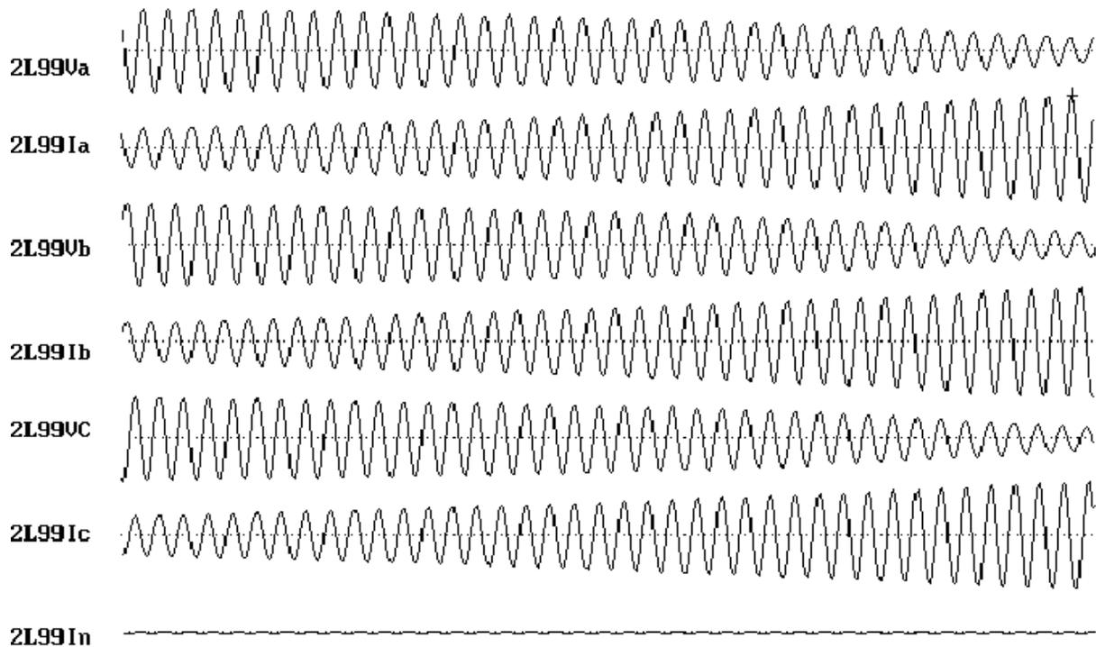
Figure E1 Digital Fault Record of an OOS Condition
