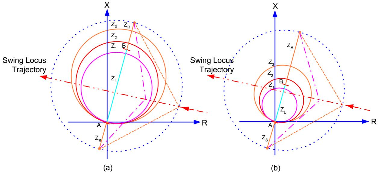
**Figure 10** Effects of Source and Line Impedance on the PSB Function
