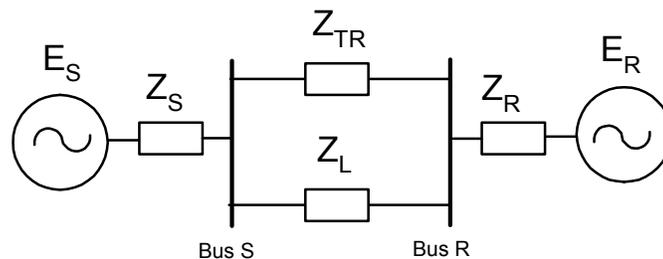
Figure 12 Two-Source System Equivalent
