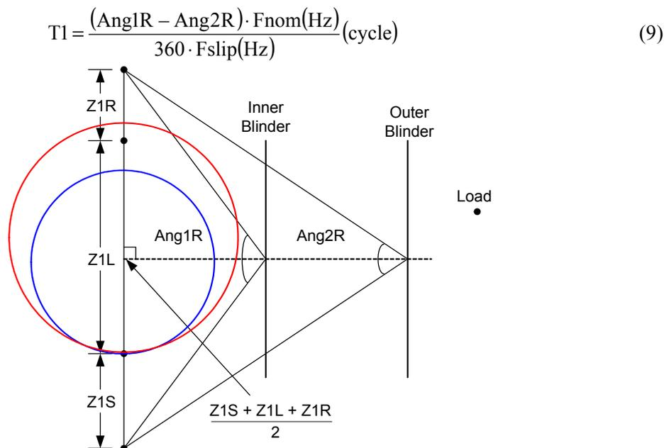
**Figure 11** Equivalent Two-Source Machine Angles During OOS
