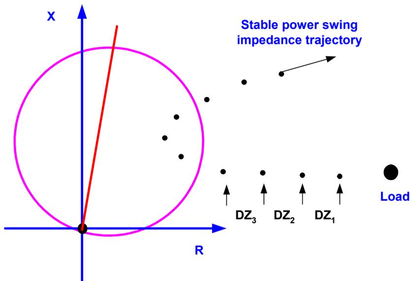
**Figure 7** Power swing detection with continuous impedance calculation
