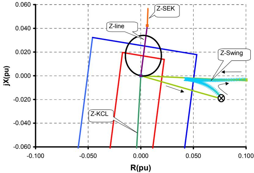
Figure B2 R-X Diagram of KCL-SEK Interconnection with Stable Power Swing Superimposed
