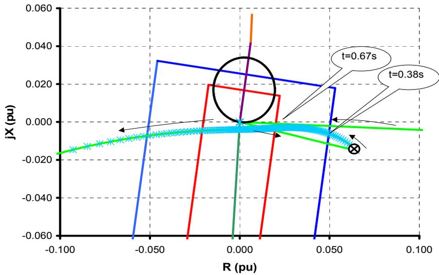
Figure B3 R-X Diagram of KCL-SEK Interconnection with Unstable Power Swing Superimposed
