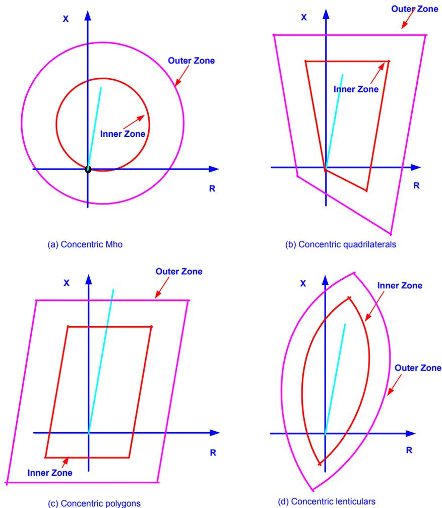
**Figure 4** PSB and OST Concentric Distance Relay Characteristics
