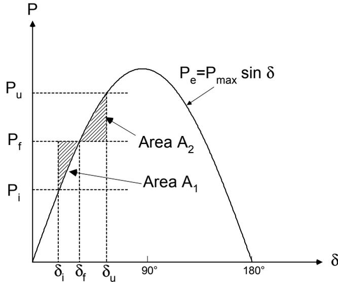
**Figure D2** Step Change in the Rotor Angle
