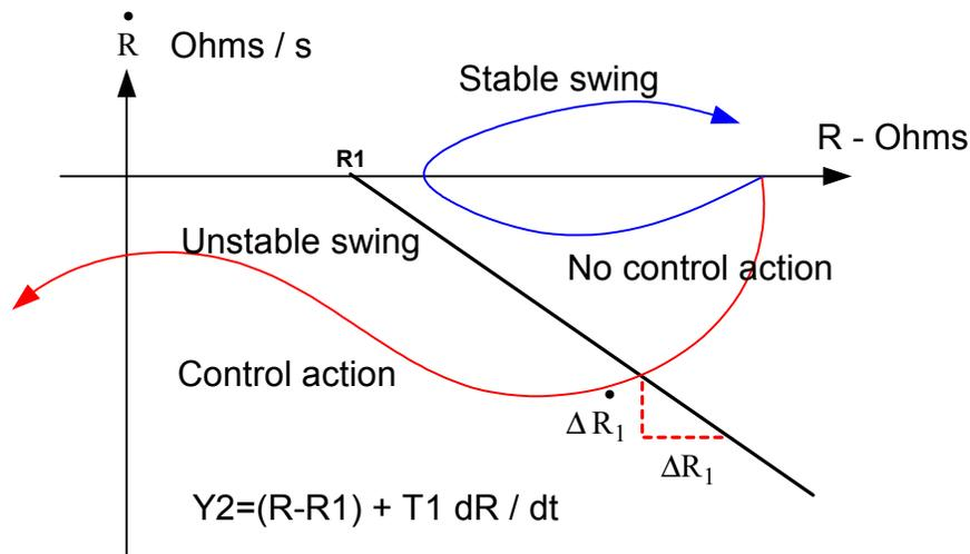
**Figure 6** Phase-plane Diagram Illustrating the Concept of R-dot Principle
