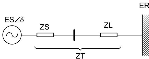
**Figure D1** Generator Connected to an Infinite Bus
