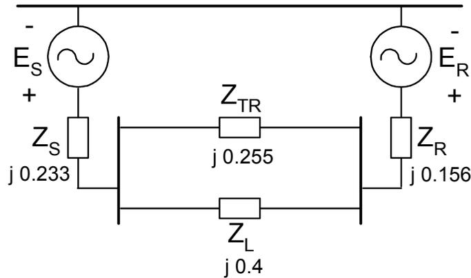
**Figure A4** Equivalent Network Between Buses 2 & 3
