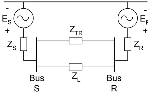
**Figure A1** Two-Source System Equivalent
