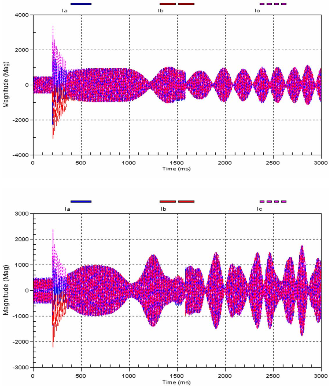
Figure 16 Typical OOS Waveforms from EMT/ATP Simulations
