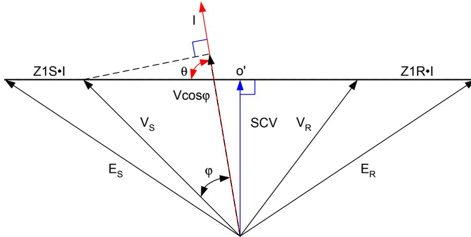
**Figure 9**  $V \cos \phi$  is a Projection of Local Voltage,  $V_s$ , Onto Local Current,  $I$
