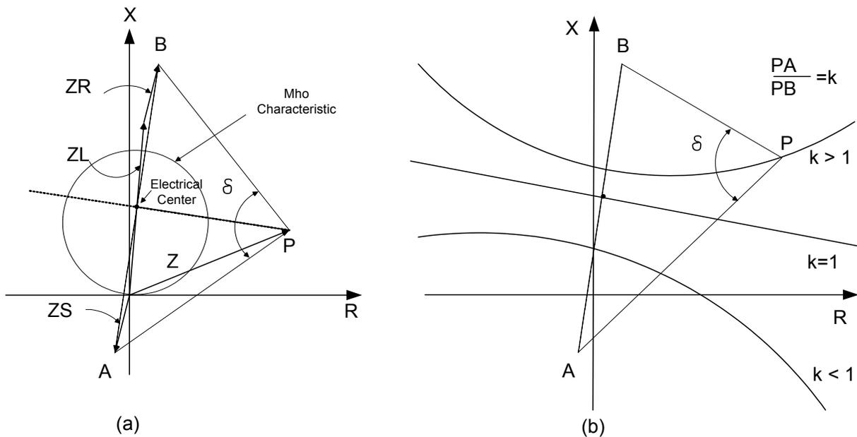
**Figure 3** Impedance trajectories at the Relay During a Power Swing for Different  $k$  Values
