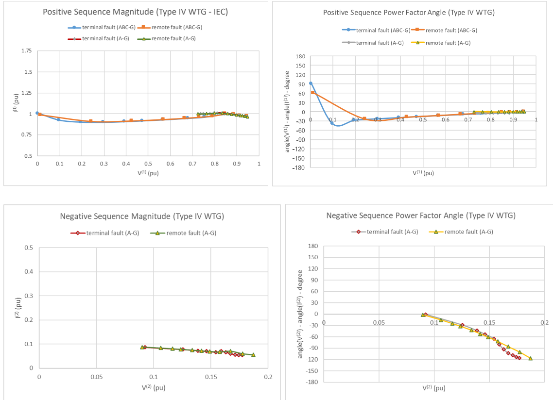
Fig. A.2-5. Magnitudes and power factor angle of Type-IV WTG modeled as per IEC Standard 61400-27-1, after one cycle.
