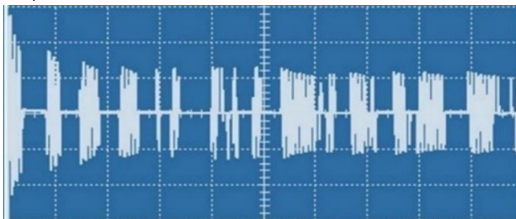
Figure 5.1 Example of intermittent and harmonic-rich HIF current waveform.
