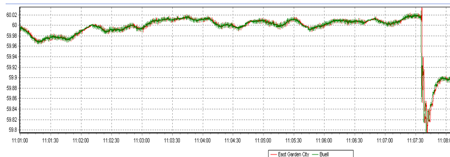
Figure B.4: BPA Synchrophasor data plot frequency excursion at transmission voltages
