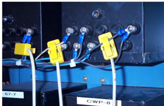
Figure-1; Non-Intrusive, clamp-on, Hall Effect Sensors
