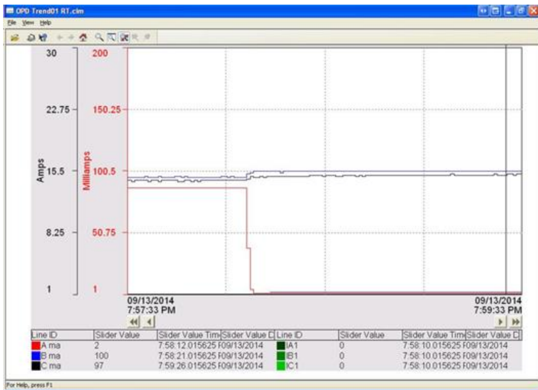
Fig. G-3. Lab data from “A”-phase open test case.
