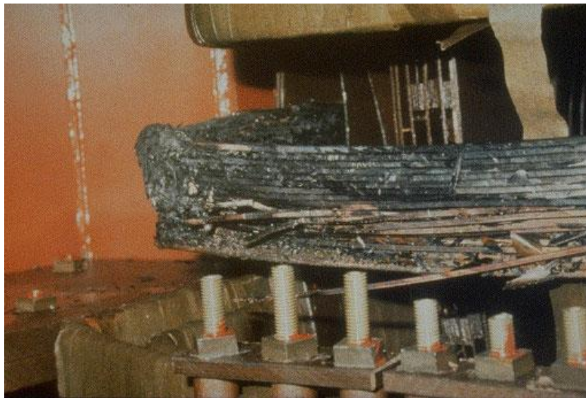
Fig. 1-8 Transformer damaged at Salem Unit 1, year 1989 (Photo Courtesy of PSE&G)
