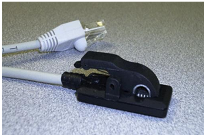
Figure 4-2 Hall-effect ECT with Shielded Clothespin Enclosure
