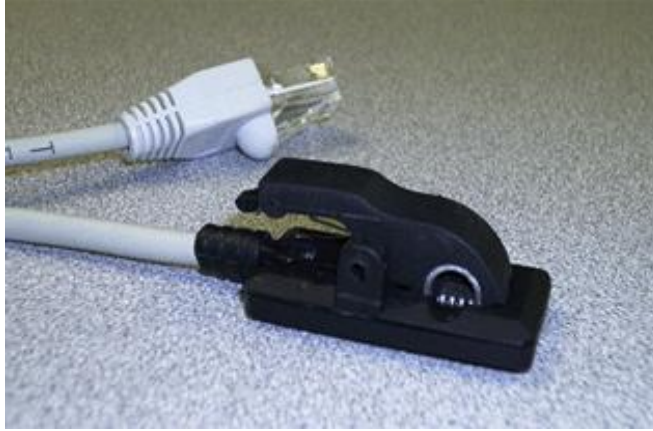
Figure 5.6: Hall-effect ECT Sensor with Shielded Clothespin Enclosure
